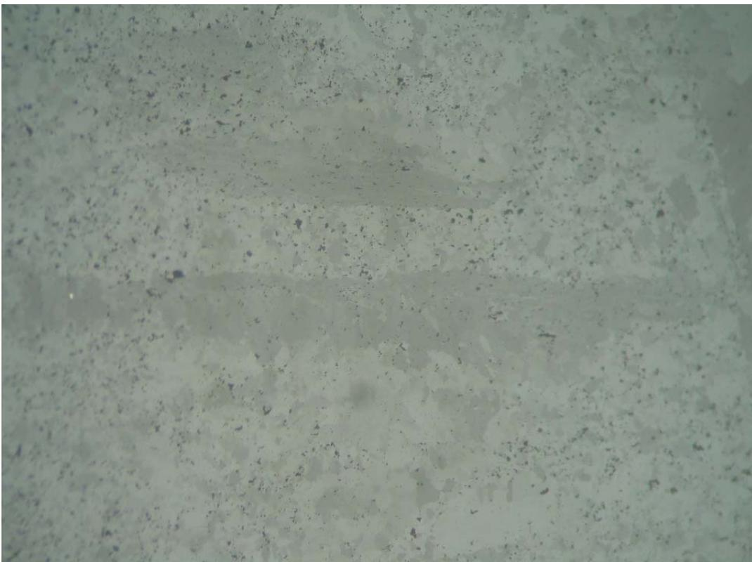
Figures 3 and 4. Microscopic view of the gray limestone. It is showed an incipient recrystallization.
